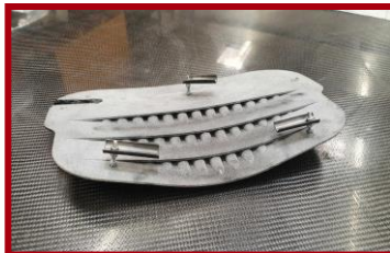
[Air duct, printed on large HSS printer]
