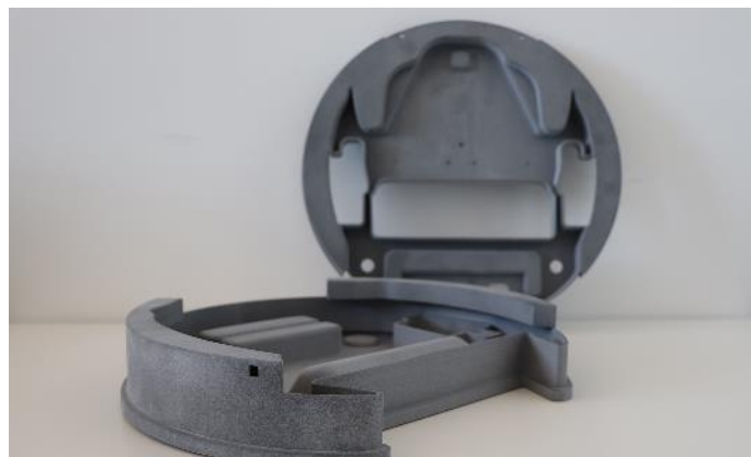
[Vacuum cleaner robot housing, printed on large HSS printer]
