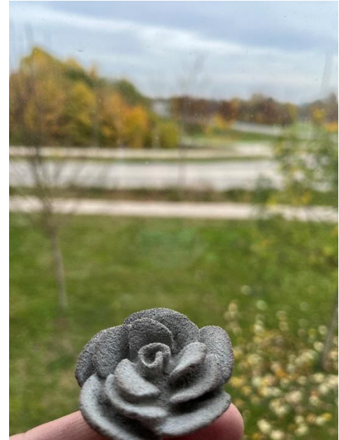
Directly printed in concrete; complete „as-is“ out of the printer, no post-treatment
