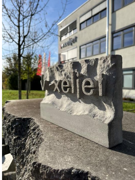
Directly printed in concrete; complete „as-is“ out of the printer, no post-treatment
