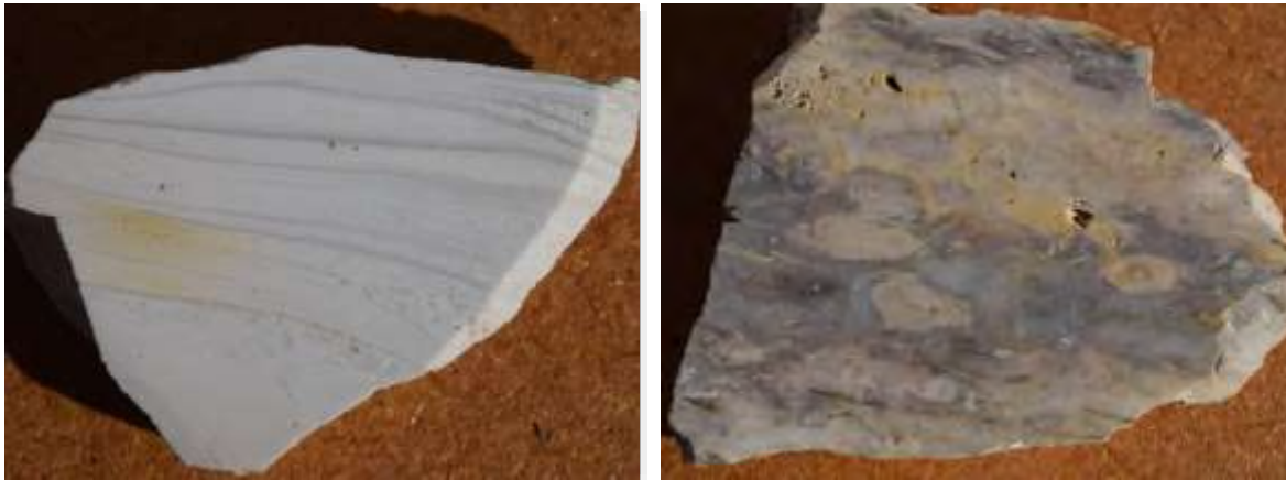
Figure 7-6 Chalcedonic Sinter Overlaying the Gravel Creek Deposit (sample widths are ~10 cm)
