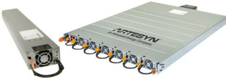
Traditionally, data center racks have used 12-volt power shelves, but higher performance compute and storage platforms demand more power, which results in very high current. Moving from 12-volt to 48-volt power distribution reduces the current draw by a factor of four and reduces conduction losses by a factor of 16. This results in significantly better thermal performance, smaller busbars and increased efficiency.
