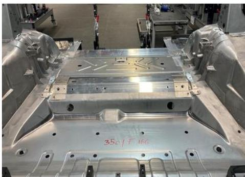
*Rear Floor Assembly – Cast Aluminum*
